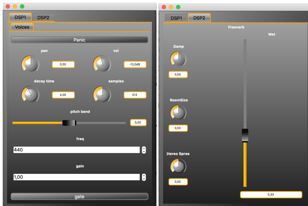
Figure 10.2: Polyphonic instrument with output effect GUI interface: left tab window shows the polyphonic instrument with its Voices group only, right tab window shows the output effect.
