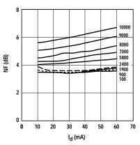
Figure 12. NF vs. I<sub>d</sub> and Frequency (MHz).
