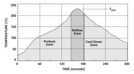
Figure 12. Surface Mount Assembly Profile.
