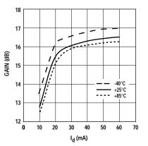
Figure 2. Gain vs. I<sub>d</sub> and Temperature at 2 GHz.
