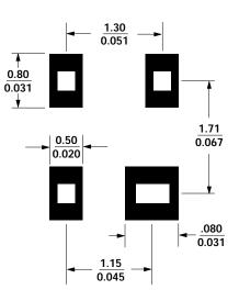
Figure 2. PCB Pad Layout for MSA-2643. Package dimensions in mm/inches.
