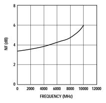
Figure 7. Noise Figure vs. Frequency at I<sub>d</sub> = 27 mA.
