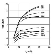
Figure 13. P1dB vs. I<sub>d</sub> and Frequency (MHz).
