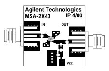
Figure 6. Complete 1.9 GHz Amplifier.
