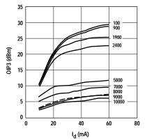
Figure 10. OIP3 vs. I<sub>d</sub> and Frequency (MHz).
