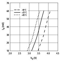
Figure 1. I<sub>d</sub> vs. V<sub>d</sub> and Temperature.
