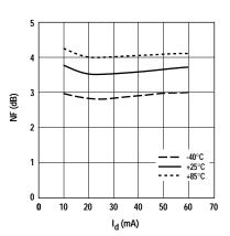
Figure 3. NF vs. Id and Temperature at 2 GHz.
