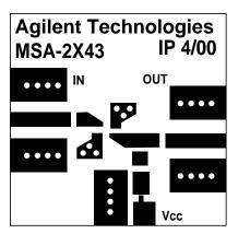
Figure 3. Multi-purpose Evaluation Board.
