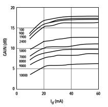
Figure 11. Gain vs. I<sub>d</sub> and Frequency (MHz).
