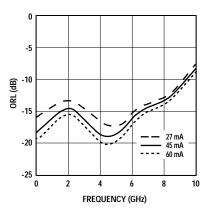
Figure 15. Output Return Loss vs. Frequency and  $\mathbf{I}_{\mathrm{d}}.$
