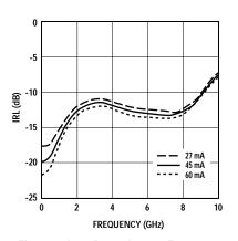
Figure 14. Input Return Loss vs. Frequency and  $\mathbf{I}_{d}.$
