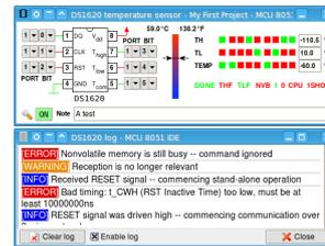
**Figure 6.1:** DS1620 simulator and its log window
