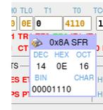
Figure 3.7: Representation of a register value in various numeric bases
