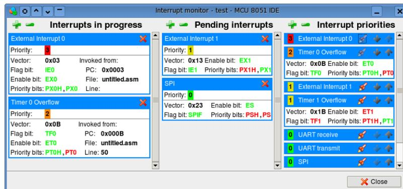
Figure 3.26: Interrupt monitor
