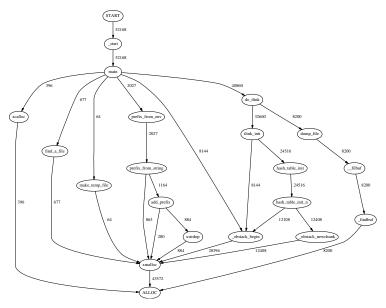
The allocation call graph for the prelinker, collect2, is a lot simpler than the previous graphs. There are no cycles in the graph and most of the allocations are concerned with maintaining hash tables. Once again, xmalloc() and \_obstack\_begin() are the two main sources of memory allocation.
