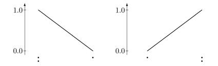
Figure 2.2: Linear B-splines of with multiple knots at one end.
